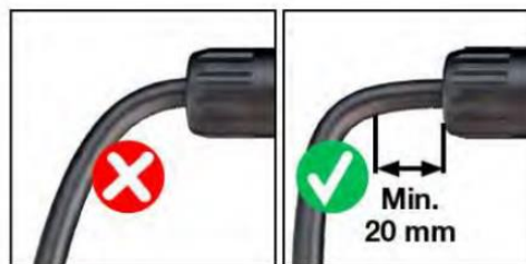
Figure 5-8 Cable routing
